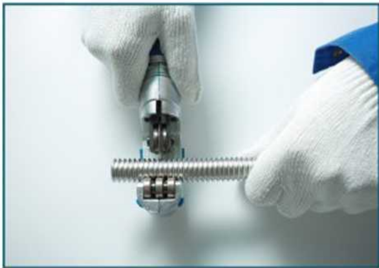
cut the pipe
